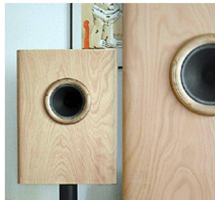
The speaker sports not merely an open back (which allows you to look directly into the back of the driver), but beautifully curved side vents which channel (but do not amplify) part of the back wave to the sides of the speaker.
